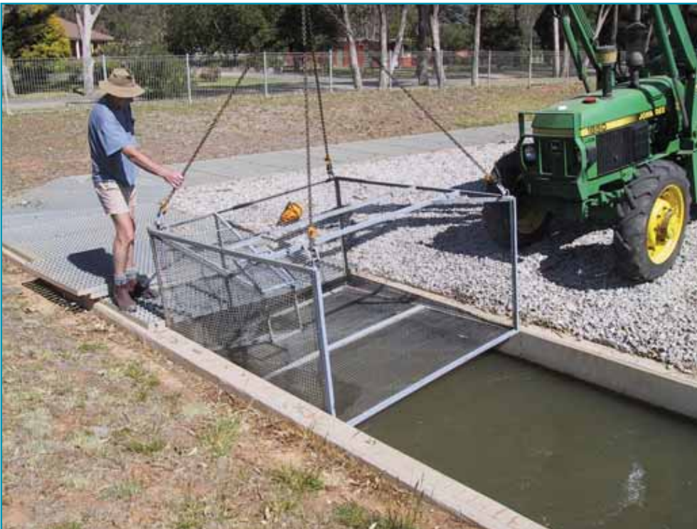
Crane lifting prototype carp separation cage at Torrumbarry Weir
